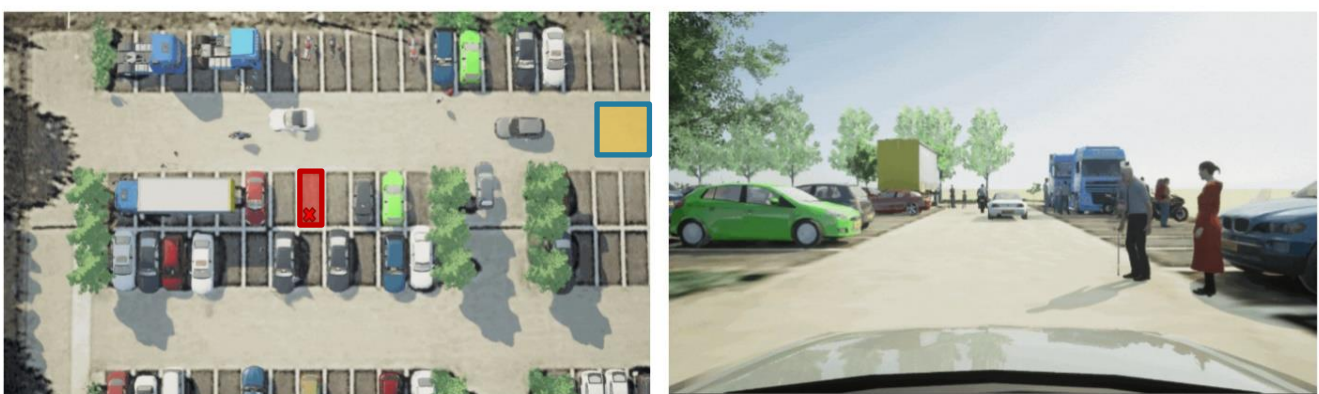
Figure 2: An example of our targeted Operational Design Domain (ODD) including dynamic road users and potentially varying weather conditions. The left image shows a bird's eye view with the drop-off zone in yellow and the designated parking slot in red. The right image shows a driving view, highlighting a pair of pedestrians at risk.
